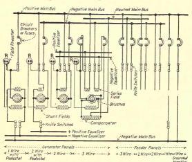
Fig. 212.—Typical low-voltage, direct-current, switch-board connections.
